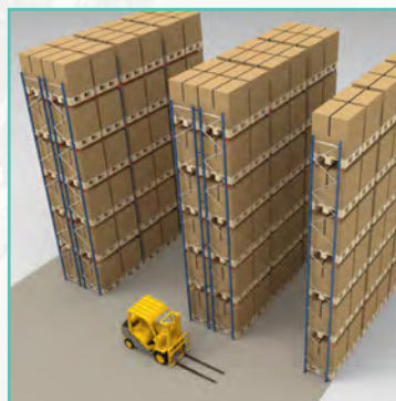
Selective Pallet Racking System
