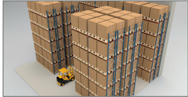
Double Deep Racking System
